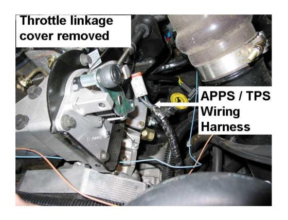
Open the loom and locate the Light Blue w/Black wire and install a supplied Posi-Tap™ to it. When locating the wire refer to the APPS pinout below. Pin location for the wire is APPS Pin 3.
